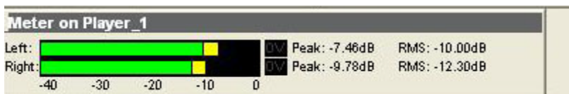
Figure 2. A stereo peak meter display. The RMS is the green bar and the peak is the yellow bar.
