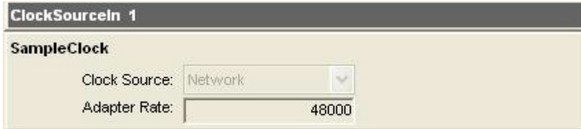
Figure 6. Clock Source information for CobraNet devices as seen in ASIControl.
