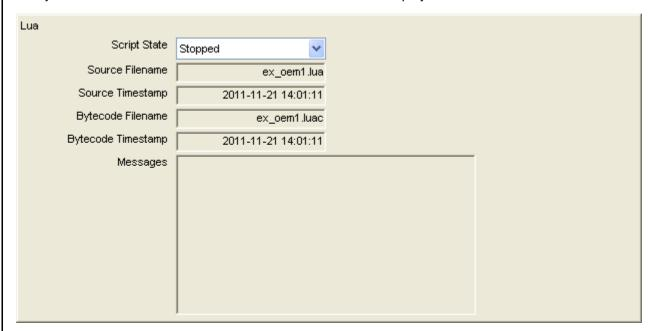
Most lua control block functions are obvious. The Script Status option is used to control the script status and the Messages section shows message from the lua runtime engine running on the network node. If a script is selected to be run, the setting will be preserved through a power down cycle of the network interface.
