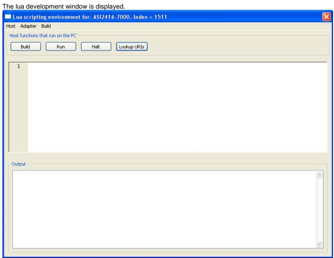
Starting from the top left we have a "File" menu for loading and saving lua source files to and from the host PC hard-drive. Next we have the "Adapter" menu which operates the device's lua file storage. It supports saving lua source files and lua byte code to the network interface.
