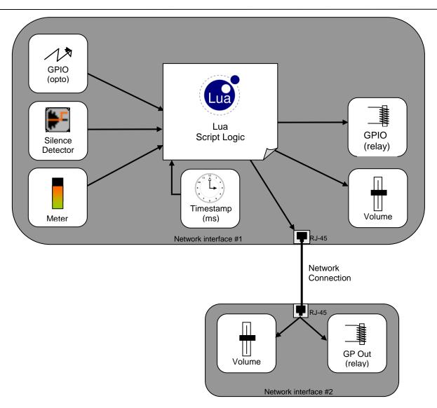
Figure 1. Inputs and outputs to and from a lua script on an AudioScience network interface
