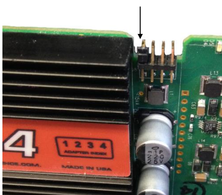
Adapter Jumper set to Adapter #1
