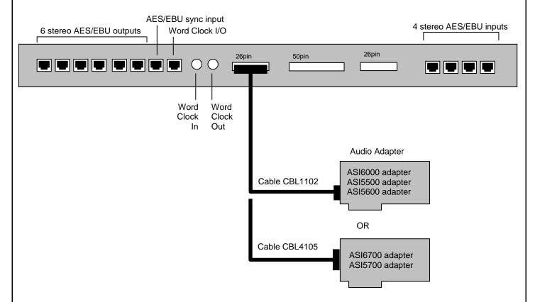
**NOTE**: On ASI6518 or ASI6618 sound cards, AES inputs 3 and 4 can be assigned as outputs 7 and 8. This allows one HUB-12 to be used; it will then have 8 AES/EBU 'outputs'. Please refer to the ASI6518/ASI6618 datasheet for further information on how to set this up.
