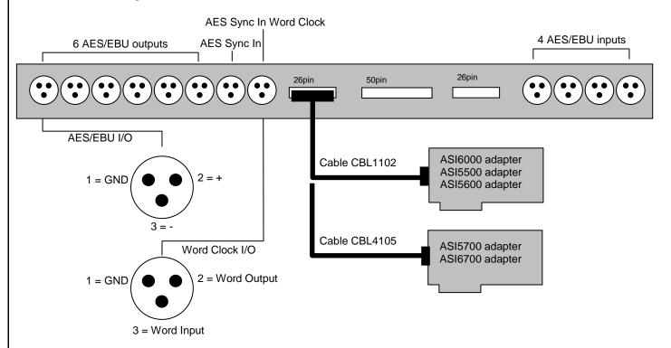
**NOTE**: On ASI6518 or ASI6618 sound cards, AES inputs 3 and 4 can be assigned as outputs 7 and 8. This allows one BOB1024 to be used; it will then have 8 AES/EBU 'outputs'. Please refer to the ASI6518/ASI6618 datasheet for further information on how to set this up. Gender changers will be needed to make BOB1024 inputs 3 and 4 correctly gendered to become outputs. <end>
